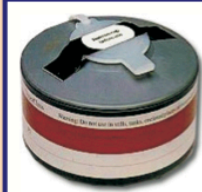
RP/02G The combination of particle filter type P3 and of activated carbon gas filter of Class-A2 for the filtering of organic vapours, gases (solvents) and particles, A2P3
